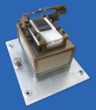
ZIF Socket provides easy load and un-load of packages
